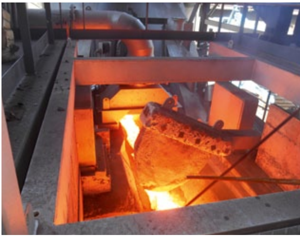
Flow of slag to the granulator Photo: Primetals Technologies Austria GmbH
