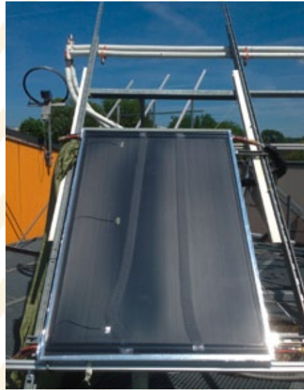
SolPol collector on the solar testbed Photo: AEE INTEC
