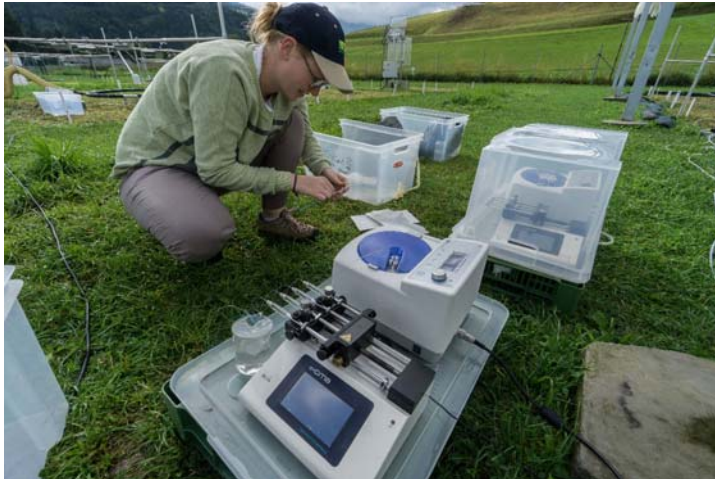
Figure 5 Usage of the microdialysis device in the field (Photo credit: Erich Pötsch)
