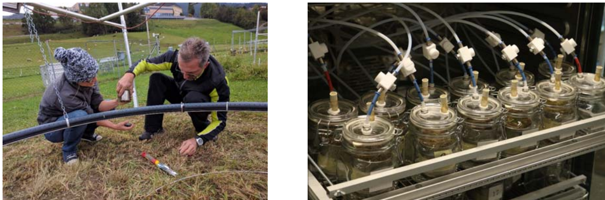
Figure 3 Sampling of intact soil cores (left side) and incubation in Kilnar jars (right side) for experiment 1a Photo credit: Evi Deltedesco.
