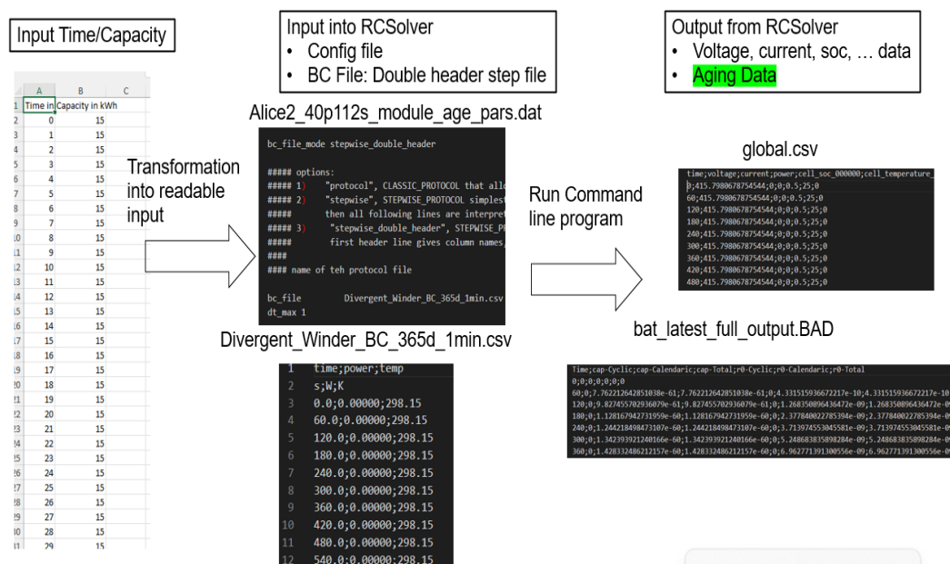
Figure 11: Virtual Vehicle workflow for battery aging simulation using RCSolver.
